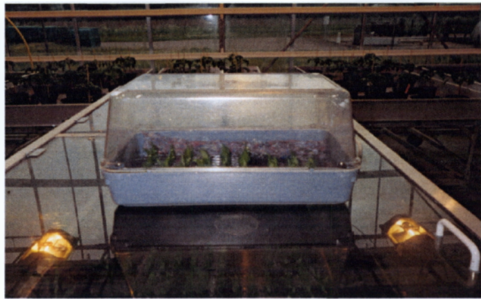
Picture 5: Small plastic container. The small plastic container consist of two parts, the upper part (transparent) and lower part (with dark gray color). The previously described trays were incubated in the plastic container on a carpet soaked with water.
