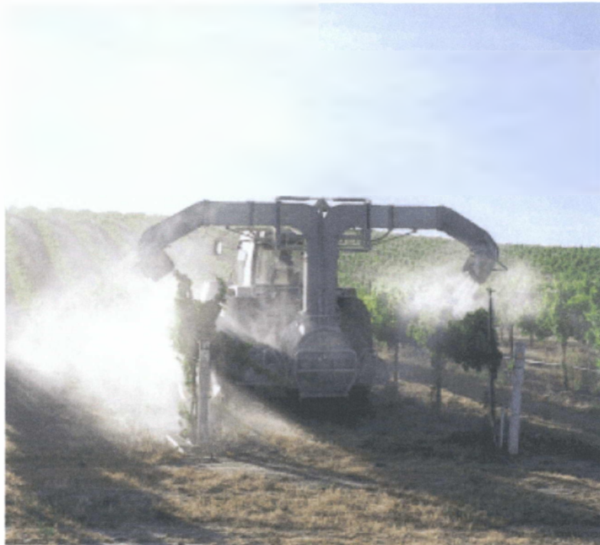
Electrostatic two-row sprayer.
