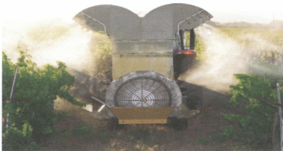
High volume (30 to 200 gallons per acre) air blast sprayer.
