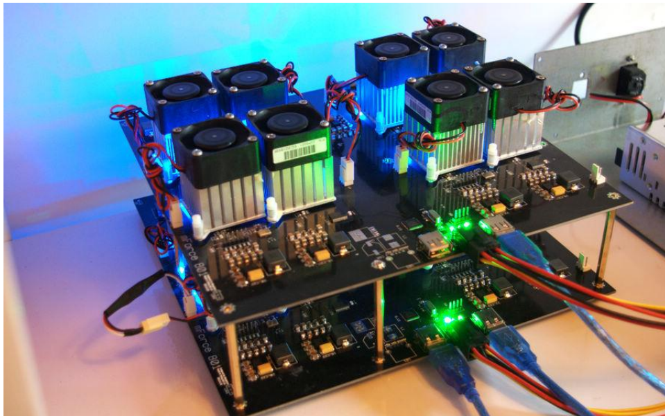
(8 cores fpga bitcoin miner)
